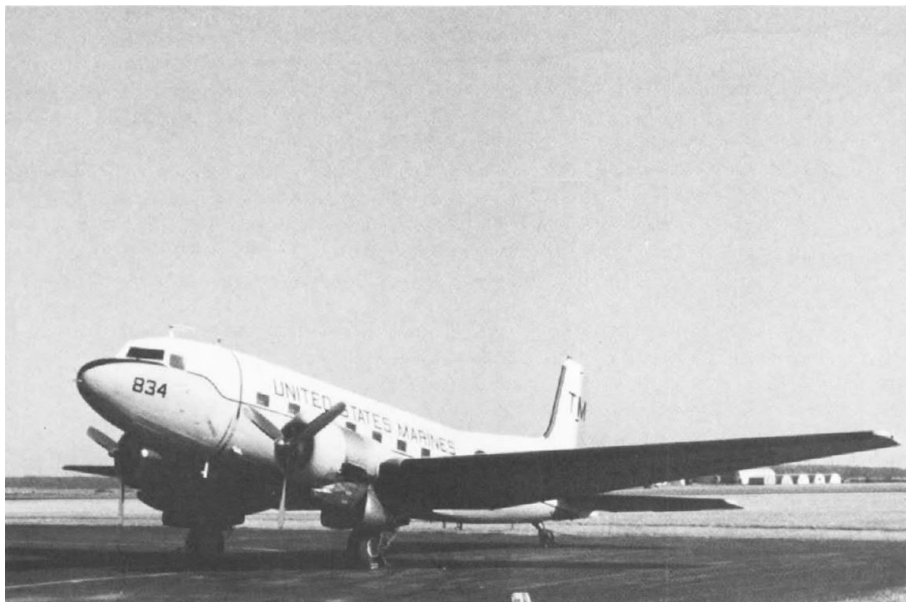
Douglas' R4D-8, the military version of its Super DC-3, entered service with the Marine Corps in 1951. In 1962 this model in the Skytrain series was redesignated the C-117D.
